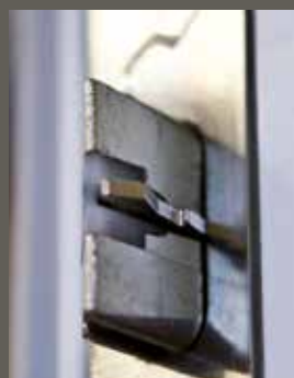
The two bars move automatically forward and hold the door in place.
