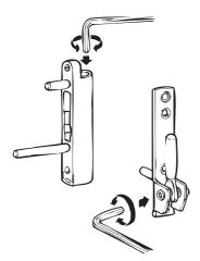
Adjust sash pressure against the weather strip by turning the sash pin.
