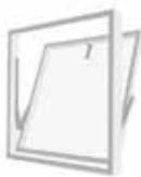
Horizontal pivot – seen from the inside
